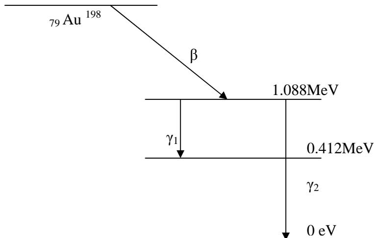
12. Find the energy corresponding to the emissions  $\gamma_2$  and  $\gamma_1$  in the diagram shown. Also predict the nucleus formed after the  $\beta$  decay.
